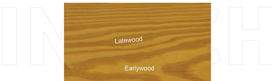
Figure 1. Image of flat-grained southern yellow pine wood showing distinctive wide earlywood and latewood sections.
